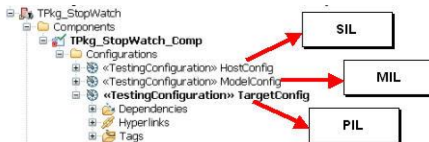
Figure 42: Configurations for MiL (ModelConfig), SiL (HostConfig”, and PiL (TargetConfig) execution.
